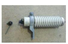
DFA technology enabled detection and identification of a failed arrester, thereby improving response.
