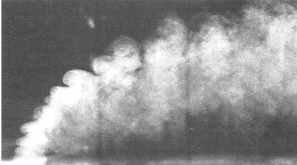
Figure 8. Photograph of laboratory study of a vertical turbulent jet in a cross wind. 13 The cross wind flow is from left to right.
