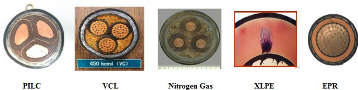
Exhibit 4.15.1 Underground System Cable Types
