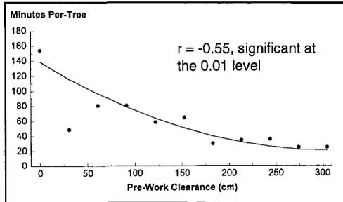
**Figure 4. Relationship between proximity to the conductors and time (worker-minutes) to prune trees at utility C.**
